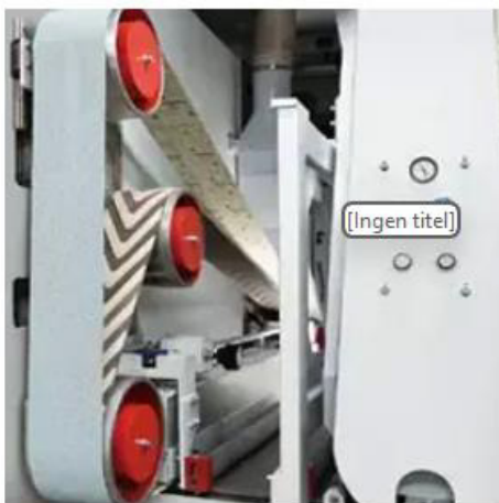
Equipped with a herringbone belt (4710mmx140mm) ,for the high gloss and skin feel sanding effect.
