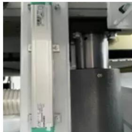
MBS full closed loop positioning system Repeat positioning accuracy increased by more than 25 times.
