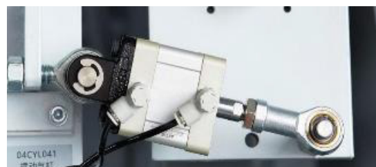
Belt oscillation: The advanced device for the sanding belt oscillation, make it easy and convenient to adjust correct oscillation.
