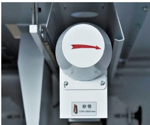
Air jet cleaning: The effective air jet cleaning of the sanding belts together with the hood that collect the dusts, prevent a dusty sanding machine and
