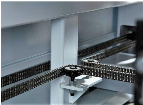
Lifting up: The double row chain minimizes deviations of the lifting structure, caused by stretching by the chain. prolong the lifetime by 3 times.
