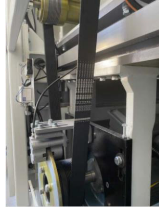
German Optibelt brand : Poly V-belt Compared with traditional V-belts, the transmission is more precise and the effect is higher. The price is more than 10 times that of ordinary triangle belts
