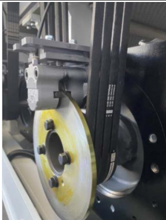
Brake: can stop with in 4 seconds
