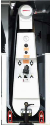
Sandpaper length 1350*2620mm To prolong the life the sandpaper and improve the heat dissipation of sandpaper
