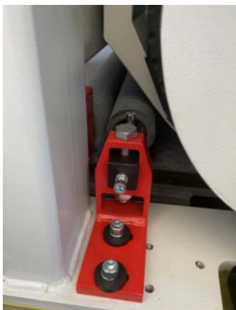
Pressure roller that can be pressed tightly when the plate passes through, rectangular spring, easy to adjust
