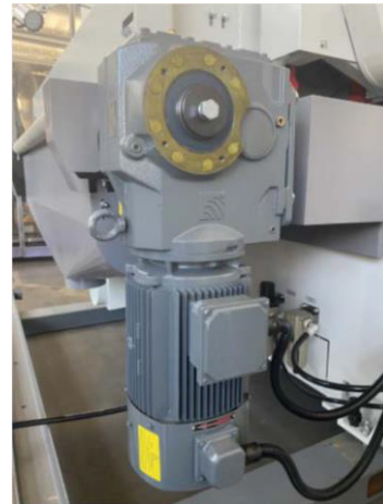
Helical gear reducer, has the highest transmission efficiency and improves transmission torque
