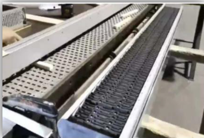
Segmented pad --- 80 pads, each pad width 16mm. Smaller pad, more accuracy
