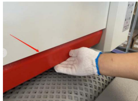
Safety automatic board to protect workers If man hand entry, the machine will automatically shut down
