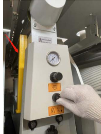
Adjustable tension pressure control. Different pressures can be adjusted according to sand belts of different materials.
