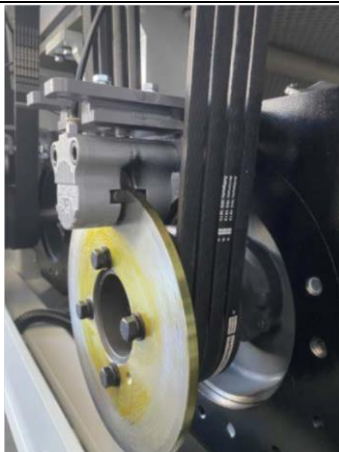
Brake: can stop with in 4 seconds
