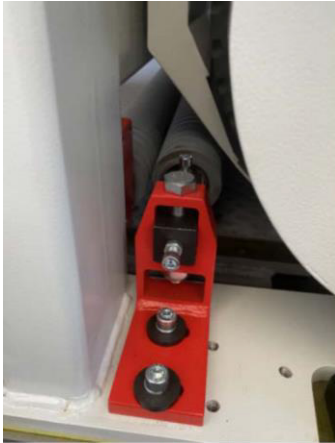
Pressure roller that can be pressed tightly when the plate passes through, rectangular spring, easy to adjust
