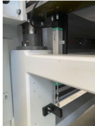
The lifting system adopts the MBS full closed-loop positioning system, and the positioning accuracy is extremely high. It is 25 times that of ordinary threaded screw, high-precision digital display detection height, display accuracy of 0.01mm.
