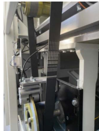
German Optibelt brand : Poly V-belt Compared with traditional V-belts, the transmission is more precise and the effect is higher. The price is more than 10 times that of ordinary triangle belts
