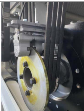
Tension cylinder + limit switch It is with belt break age protection function
