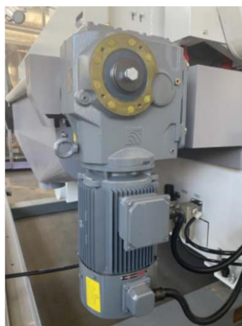
Helical gear reducer, has the highest transmission efficiency and improves transmission torque
