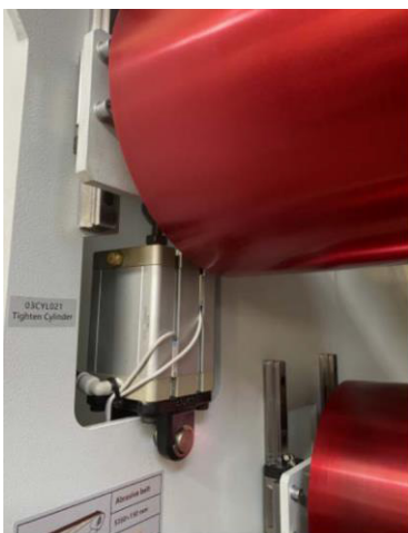
Tension cylinder + limit switch It is with belt break age protection function
