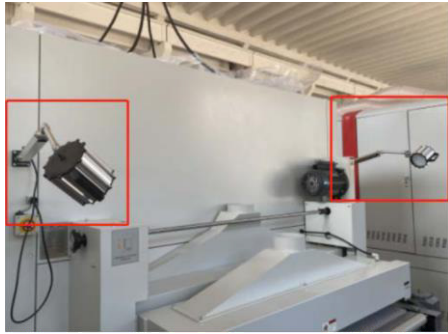
The light inspection lamp after the board comes out helps quality inspectors detect the layout effect. More user-friendly design
